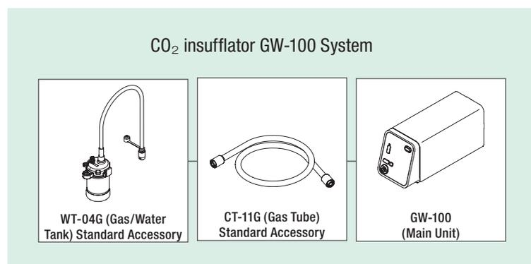
Tube sets for the connection of GW-100 to the medical gas pipeline and medical gas cylinders are available.
